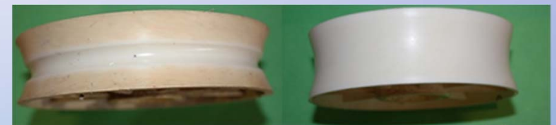
An example of an early type plastic roller showing serious grooving.
